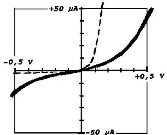
Fig. 1. Characteristic curve for the replica detector. The curve for a typical point contact germanium diode (OA81, 1N34) is shown by dotted line.
